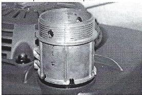
Insert a screwdriver into the drilled holes for leverage when removing or installing a fuel tank nut.
